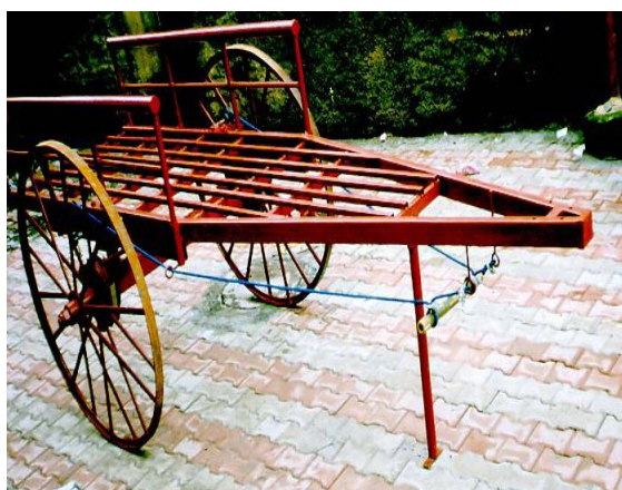
Fig 1: Photograph of two wheel steel cart (2.0 tones capacity) without rubber liner on its wheel
