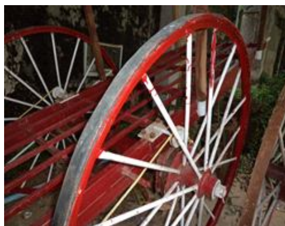
Fig 2: Photograph of two wheel steel cart (2.0 tones capacity) with rubber liner on its wheel
